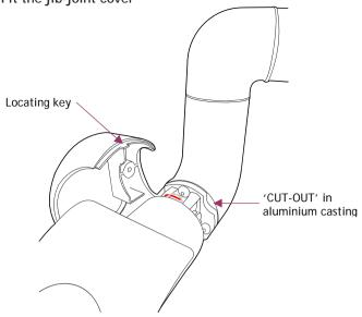
Covers are marked 'L' and 'R' on their inside faces as viewed from the end of arm. Engage the slider, with its 'T' mark uppermost, into the groove inside the cover.
