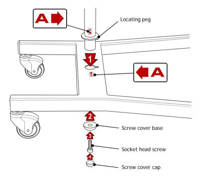
Fit the upper section of the up-stand to the lower section of the up-stand with the screw and shake-proof washer using the hex wrench provided.
