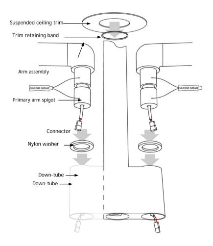
Join the connector from the primary arm to the connector from the down-tube.
