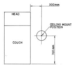
WARNING: the light-head operates from a low-voltage supply produced by a transformer in the ceiling mount assembly and fed through the suspension arm. On NO ACCOUNT should the arm be connected directly to mains voltages.
