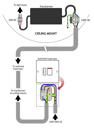
SL180LEDC wiring diagram
